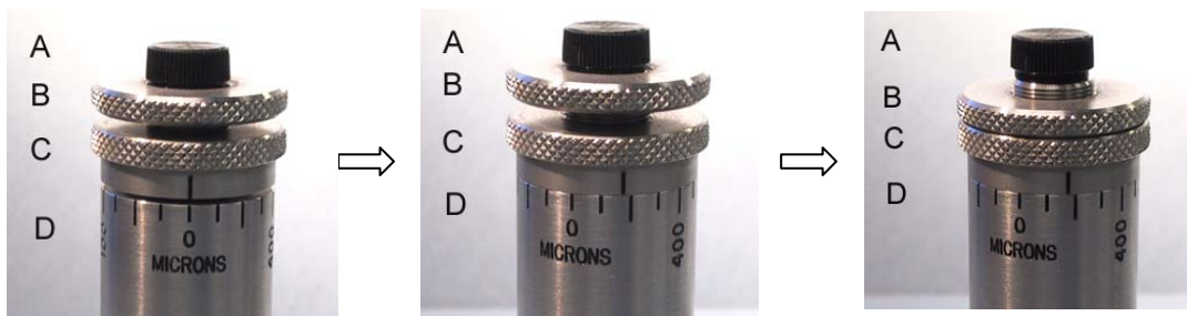
Figure 2: Images of the Model 145 micrometer dial arrangement demonstrating the zeroing process. On the left, the micrometer dial (A) is rotated counter-clockwise until there is a space between the dial and the housing (C). The locking ring (A) is also above the micrometer dial. Next, the micrometer dial is rotated clockwise until it becomes snug on the housing. This is the zero position. Finally, the locking ring is rotated clockwise to lock the position of the micrometer in place.
