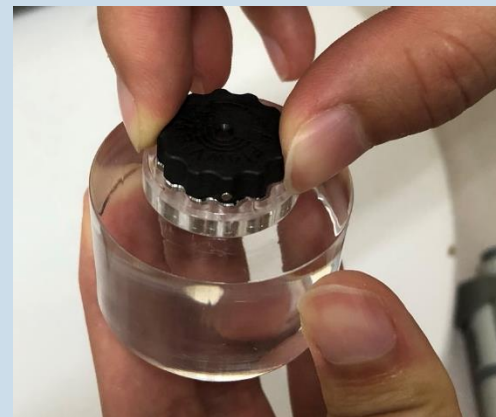
Cover holder with lid, twist slightly
