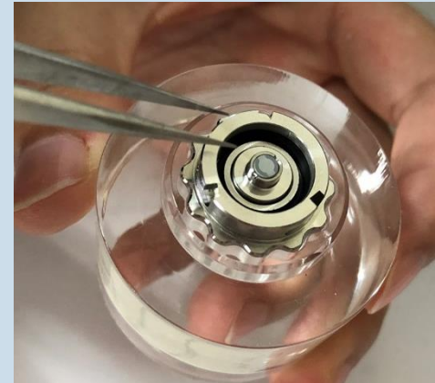
Put chip onto center of holder, align it with tangent line
