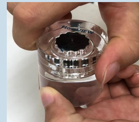
Twist acrylic case to fit holder (Make sure upper and lower lines align)
