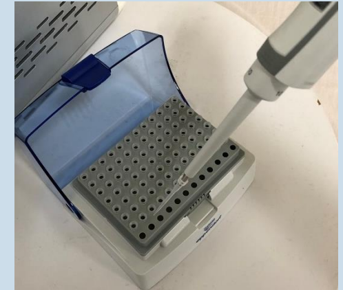
Take out pipette and install tip
