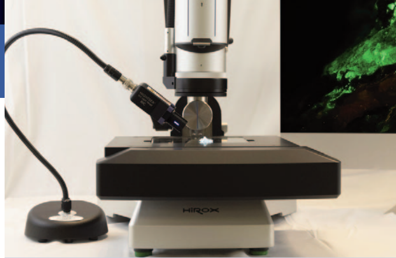
Hirox HR-1020E lens with NIGHTSEA UV illuminator
