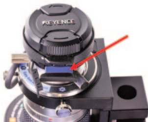
Z100, Z500, and ZST lenses – the barrier filter inserts in the Analyzer slot at the top of the lens.
