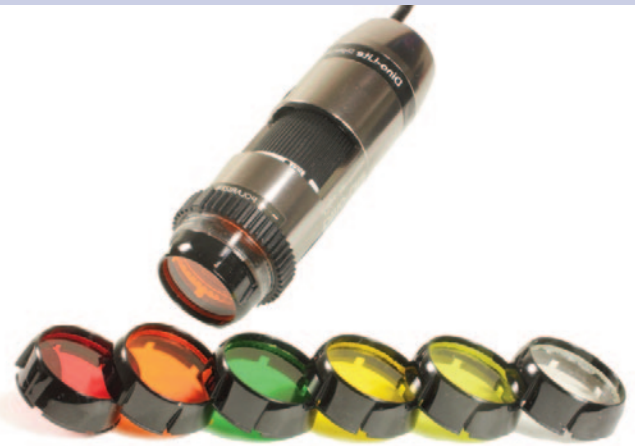
Dino-Lite digital microscope with array of NIGHTSEA barrier filters
