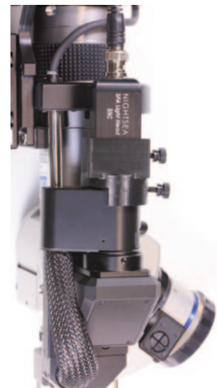
Keyence VH-ZST lens, fiber optic port with NIGHTSEA adapter and light head
