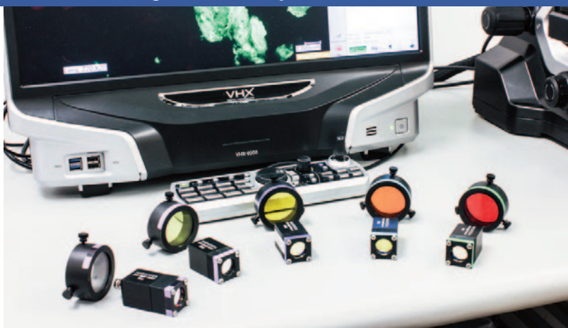
Various excitation light heads and corresponding barrier filters.
