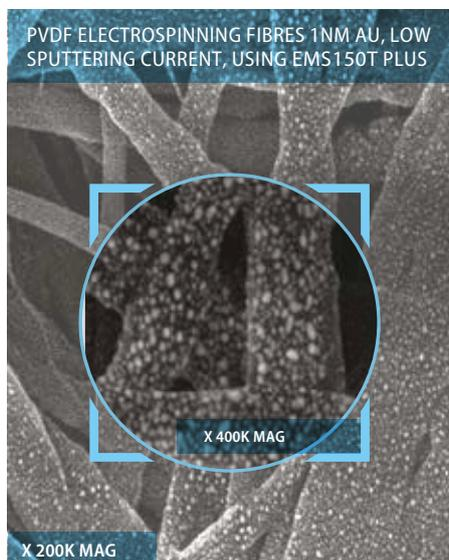
Smaller grain size allows for fibre morphology features to be seen and allows for individual fibres to be identified.
