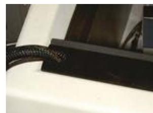
10: Adhere the cable holders along the top outer wall of the cryostat
