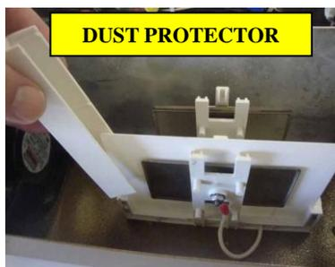
**\*NOTE: set dust protectors aside and after you clean the plates inside the machine. Reinstall them by sliding them back onto the slot that they were removed from on the back of the plate holder.**
