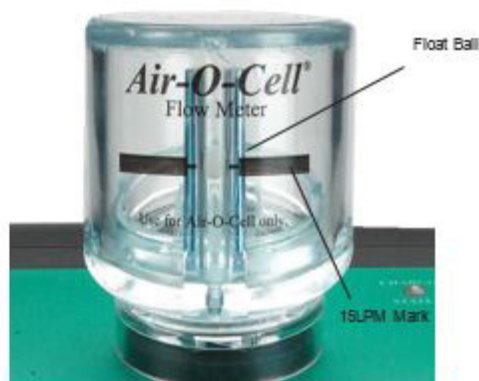
Adjust flow until ball is centered on line
