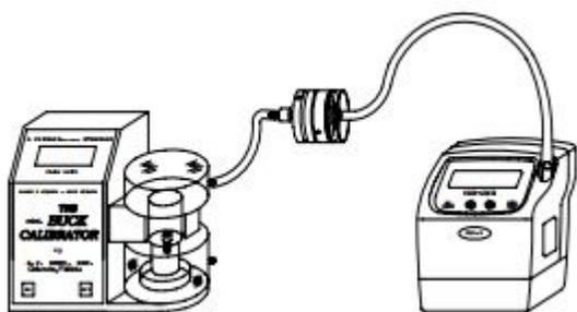
3. Wet flow cell by connecting a pump flowing at 1000 to 2000 cc/min. for Catalog #65240-61 – mini-BUCK™ (Medium Flow) and 5 LPM for #65240-63 – mini-BUCK™ (High Flow). Initiate soap film up center tube by rapidly pressing button down and releasing. Repeat this procedure until bubble doesn't break. The tube is now wet and tests at any range may be conducted. One minute warm up time is all that is required of the mini-Buck.
